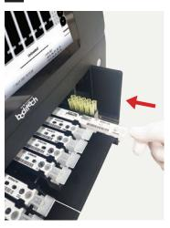
2 Insert sample tube into tube rack
